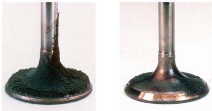
Figure 3. Comparison of intake valve deposits before and after deposit control additive use
