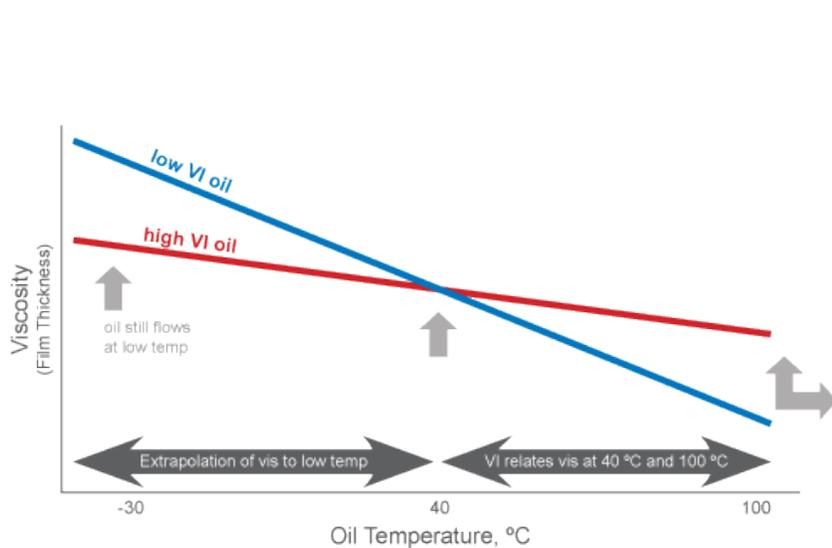
Figure 1. Oil Viscosity vs. Oil Temperature
