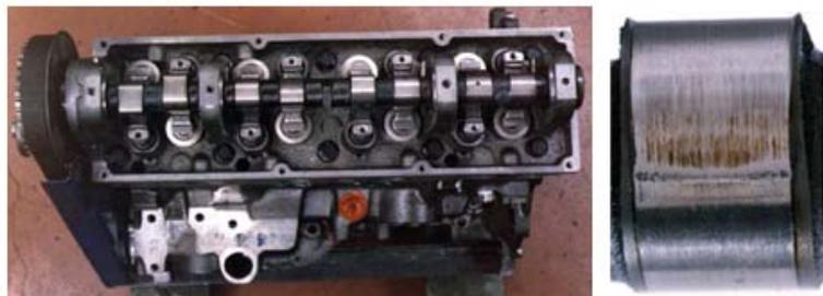
Figure 2. Example of valve train and close-up of wear on a camshaft lobe.
