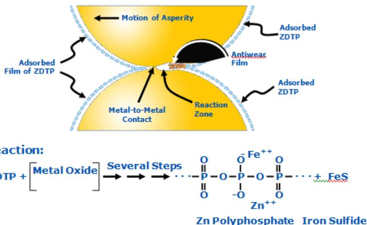
Figure 3. Creation of the protective wear film.
