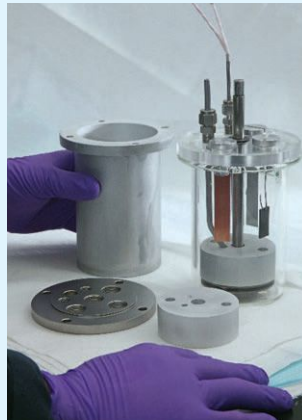
Figure 5. Setup for aluminum beaker oxidation test (ABOT). Figure courtesy of Southwest Research Institute.
