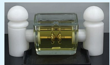
Figure 2. Dielectric breakdown testing apparatus with button electrodes. Figure courtesy of Chevron Oronite.
