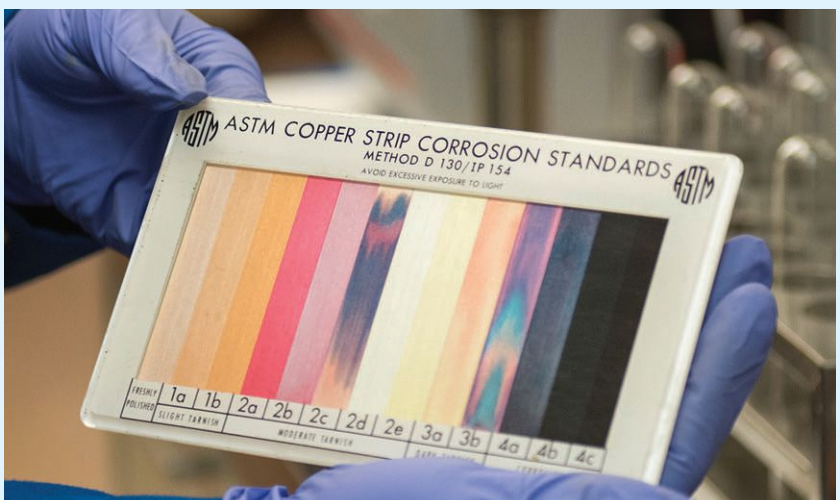
Color chart for ASTM D130 copper corrosion test. Figure courtesy of Airman 1st Class Greg Erwin, U.S. Air Force.
