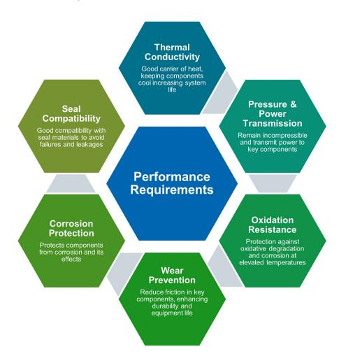
Well formulated hydraulic oils play a key role in the reliability and performance of modern hydraulic equipment, whether they are in used in industrial applications or in construction equipment. The key performance requirements that needs to be considered are: Thermal conductivity, Pressure and Power Transmission, Oxidation Resistance, Wear Protection, Corrosion Protection and Seal Compatibility, which are summarized in the Performance Requirements diagram above.
