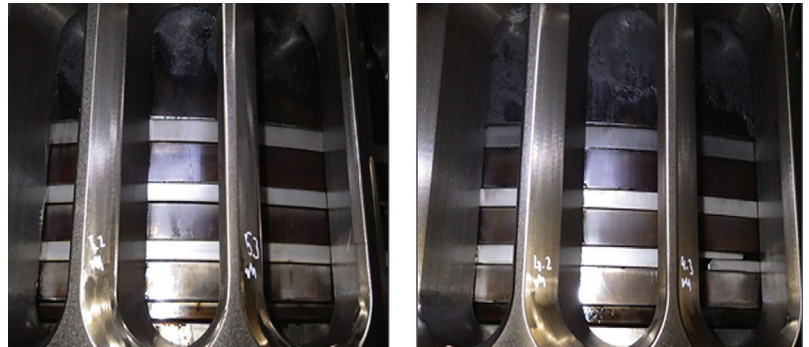
Figure 4: Cleanliness performance of 200BN and 100BN MCL
