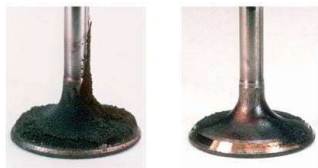
Figure 2 Intake valve deposits before and after deposit control additive use.
