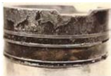
Figure 2. The heavy duty diesel piston is showing severe deposits due to lack of sulfonates.
